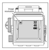
Press Mode shift button to set the camera to Playback mode and the last picture taken appears on the monitor. Press Right button to advance pictures and Left button to reverse them.
